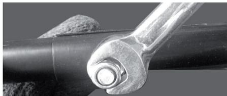
5. Slide the rubber bushing onto the end of the shaft, lining the holes in the bushing up with the holes in the shaft. The bushing has a tongue along its length which slots into a notch in the hole of the thrower housing. Slide the shaft into the thrower housing and fasten it with the two screws. **Note:** Since the mains lead runs along the inside of the shaft, you might need to hold the lead out of the way using a long slender implement to avoid puncturing it with the screws.
