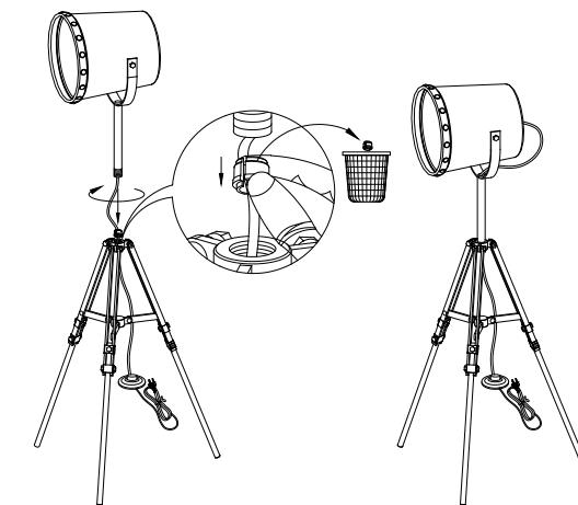
1. Screw the lamp bracket to the tripod.
