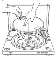
**3** Use the ribbon to hook the drive belt around the motor pulley.
