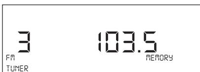
5. Press **MEMORY/CLOCK** to confirm storage of the station for the designated memory slot.
