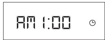
8. Confirm with **TIMER**. The display returns to the current time and **L** remains lit on the display.
