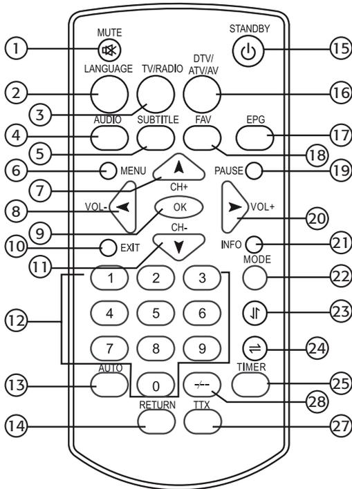
1. **[MUTE]**: Turns the sound on/off. The sound can also be reactivated by pressing V+ or V-.
