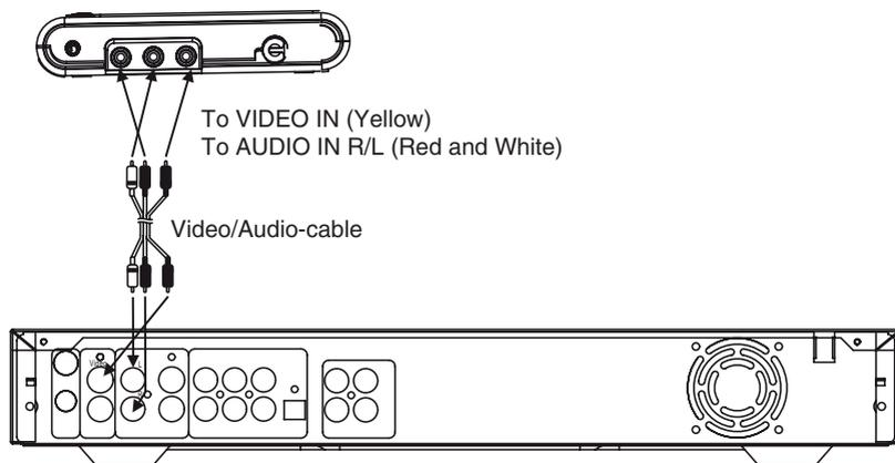
Press [DTV/ATV/AV] (16), and select AV, connect the included cable between the TV-receiver and a e.g. DVD player or digital camera. Press [DTV/ATV/AV] (16), and select AV.
