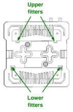
Make enough space for Zipabox on your Din-rail. Hook upper fitters on the back of your Zipabox to the Din rail and press Zipabox slightly to snap lower fitters.
