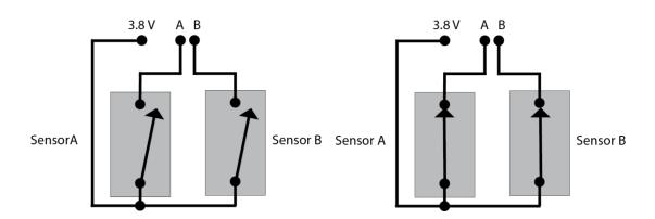
Figure 2 Two alarm sensors with closing function
