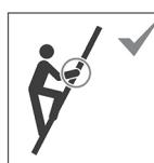
Keep a secure grip on the ladder when ascending and descending. Maintain a handhold whilst working from a ladder or take additional safety precautions if you cannot.
