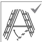
Only use the ladder with restraint devices engaged.
