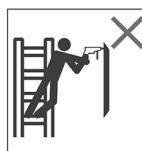
Avoid work that imposes a sideways load on ladders, such as side-on drilling through solid materials.
