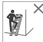
A standing ladder shall not be used as a leaning ladder unless it is designed to do so.
