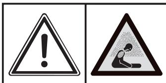
The generator must not be used indoors or in closed areas, ensure that the working area is well-ventilated.
