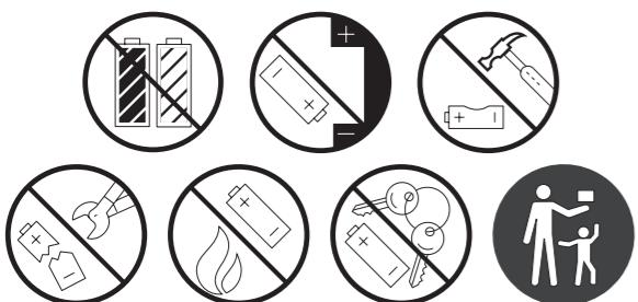
Do not mix types or brands | Insert correctly (+/-) | Do not break |
