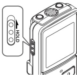
**Power on:** Slide the **HOLD** switch in the direction opposite that indicated by the arrow.
