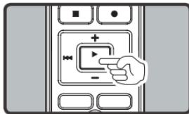
While the recorder is during playback mode, press the **PLAY/OK (▶)** button to change the playback speed.
