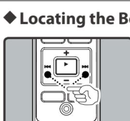
While the recorder is during playback mode (playback or playback in slow/fast mode), press the ►►I or ◀◀I button.
