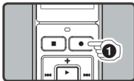
① While the recorder is during playback mode, press the **REC (●)** button at the point you want to start segment repeat playback.
