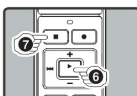
⑥ Press the **PLAY/OK (►)** button to complete the setup screen.
