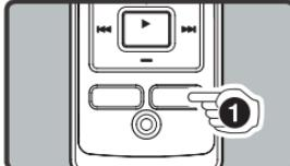
1 While the recorder is during stop mode, press and hold the DISP/MENU button for 1 second or longer.
