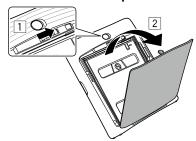
**2** Grasp the rectangular holes on the film pack and remove the empty film cartridge, and dispose.
