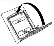
**4** A black film cover will automatically be ejected, remove and dispose.
