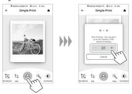
When the film has been ejected (the printer stops making a sound), hold the edge of the film and remove from the printer.
