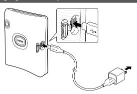
Connect the printer using the supplied USB Type-C cable to a USB AC adapter (supplied with your smartphone) then connect the USB AC adapter to an indoor power supply.
