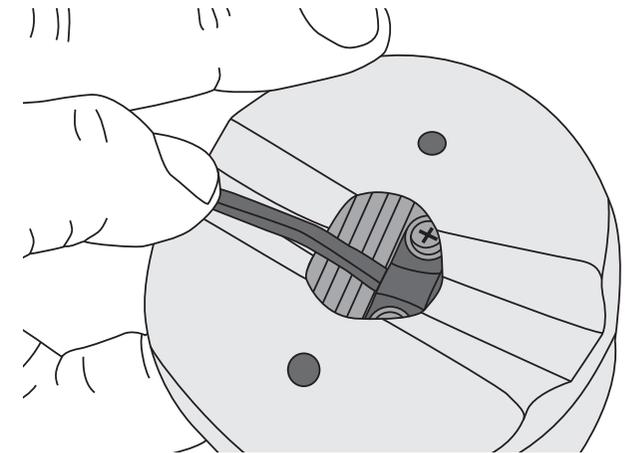
2. Ensure that the flexible cable is in the notch along the bottom of the box and fix the metal box to the ceiling using the screws provided.
