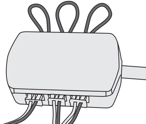
2. Lead cables and light fittings into the hole, ensure that the light fittings are properly fixed and connect the cables to the junction box.
